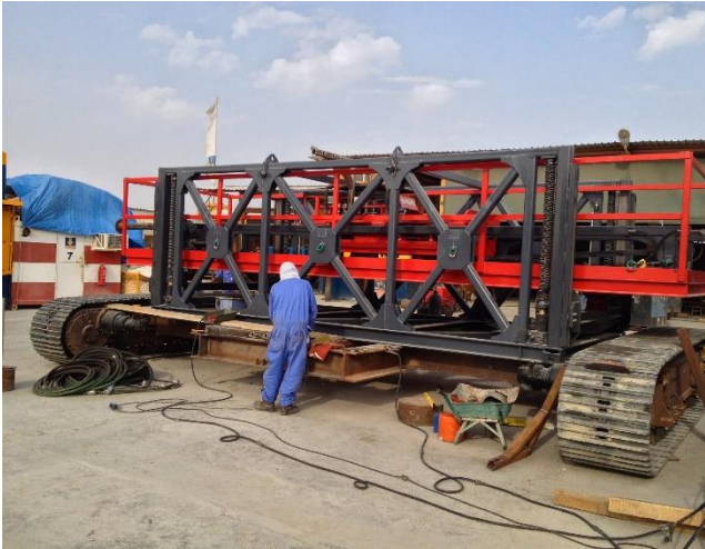
our self-built drilling rig for quick move between boreholes
