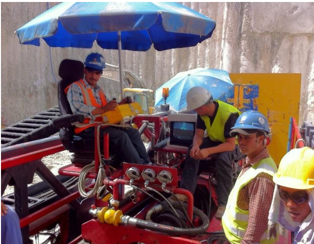
The drilling is monitored optically and by a monitor
