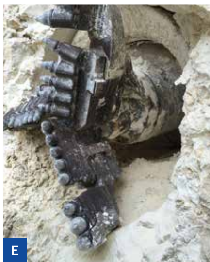
A: The Bohrtec BM600LS working on the pipe arch for tunnel 3. B: Pipe arch tunnel 1. Starting shaft. C: Pipe arch tunnel 1. Receiving shaft. D: The flat drilling head of the FS609. E: The retractable drilling head of the FS609.
