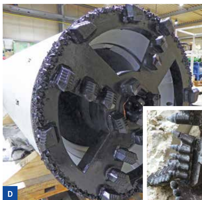
A: The Bohrtec BM600LS working on the pipe arch for tunnel 3. B: Pipe arch tunnel 1. Starting shaft. C: Pipe arch tunnel 1. Receiving shaft. D: The flat drilling head of the FS609. E: The retractable drilling head of the FS609.
